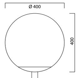
dimensions: diameter 400; weight: 4,5 kg; intendend use: top mounted luminaire; port connection: pluggable on mast cap ; material: V2A and aluminium; lamp glass: polycarbonate clear; protection rating: SkI. I (SkI. II on request); protection category: IP 54; lamp mounting: compact fluorescent light; paint work: in RAL or DB, powder coating on request; ready for connection to 230V, 50Cps
