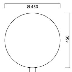
dimensions: diameter 450; weight: 4,5 kg; intendend use: top mounted luminaire; port connection: pluggable on mast cap ; material: V2A and aluminium; lamp glass: polycarbonate opal; protection rating: SkI. I (SkI. II on request); protection category: IP 54; lamp mounting: compact fluorescent light; paint work: in RAL or DB, powder coating on request; ready for connection to 230V, 50Cps
